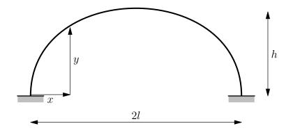
Find y(x) for an arch with horizontal width 2l and height h. Give the equations that determine the constants in your solution, but you need not solve for the constants.
