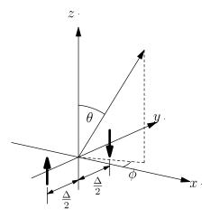
Each antenna is a center-fed dipole radiator formed from two wires, each of length  $d/2 \ll \lambda$  and driven by a current source as shown in the figure below. The wires are aligned parallel to the z axis  $(\theta = (0, \pi))$ . The current source produces a time-dependent current given by  $I(t) = I_0 e^{-i\omega t}$ . You may assume that the charge that enters the wires is uniformly distributed along their lengths.
