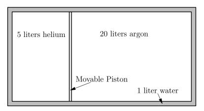
One moves the piston slowly, while maintaining thermal equilibrium, to the point where the pressure of the argon gas is twice its original value. Then, suddenly, the piston is released. The piston returns to its rest position and thermal equilibrium is restored. After the entire process the temperature of the water has increased by exactly 1.0°C. The heat capacity of water is 4.184 kJ/kg·K, and the gas constant is R = 8.314 J/mole·K.
