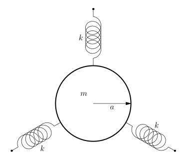
At equilibrium, the length l of the springs is greater than the relaxed length  $l_0$ . The disk remains in the initial horizontal plane but is otherwise free to move. (The diagram shows the view looking down on the plane.) What are the frequencies of the normal modes of small oscillations? What do the modes look like? Hint: You might identify the normal modes from the symmetries before calculating the frequencies.
