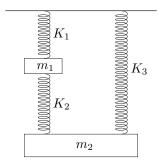
Suppose the system is oscillating around its equilibrium configuration. Find the normal modes.
