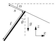
A uniform rod of length  $\ell$  and mass m moves in the x-z plane. One end of the rod is suspended from a straight rail that slopes downwards with an angle  $\alpha$  relative to the horizontal; the connection point is free to move along the rail without friction, and the rod is able to swing freely in the x-zplane. Uniform gravity acts downwards.
