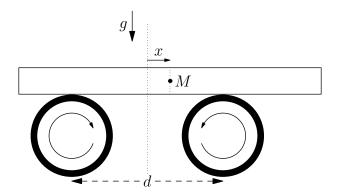
A uniform rigid slab of mass M is supported by two rapidly counter-rotating parallel horizontal rollers, with axes a distance d apart, with surfaces that brush past the slab in the directions shown in the figure. The coefficient of kinetic friction between each roller and the slab is  $\mu_k$ .
